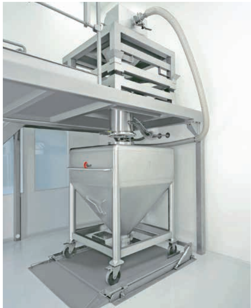
Raw material dispensing with sack discharge into an IBC
