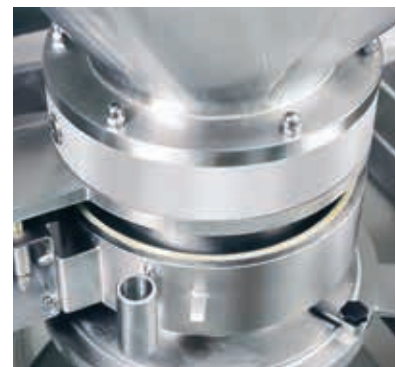
Docking system using an inflatable radial seal, docked
