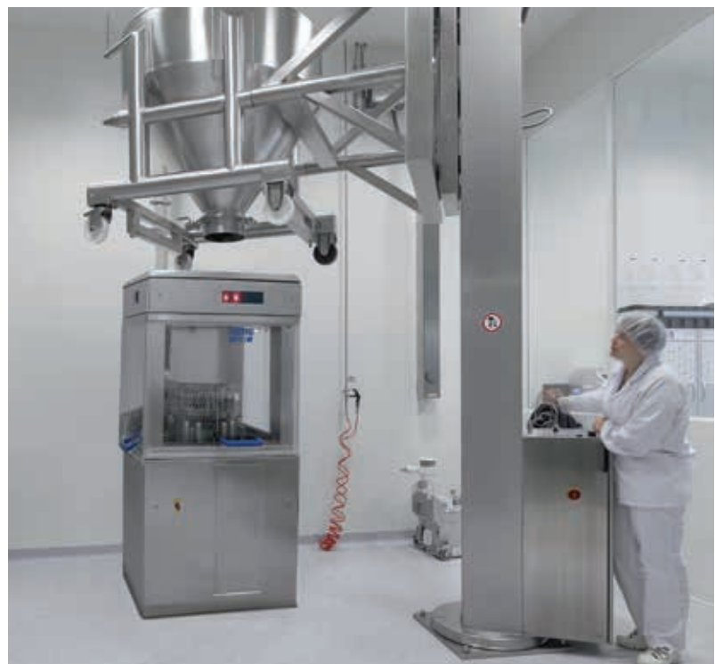
Handling equipment for product transfer from container to tablet press
