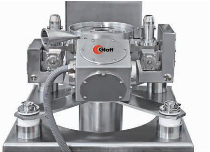
Automatic active valve half on active docking system with automatic lifting
